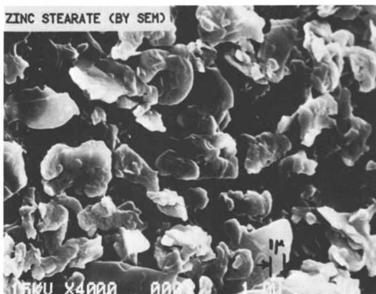
Figure 14. Scanning electron micrograph (SEM) of zinc stearate powder (technical).
